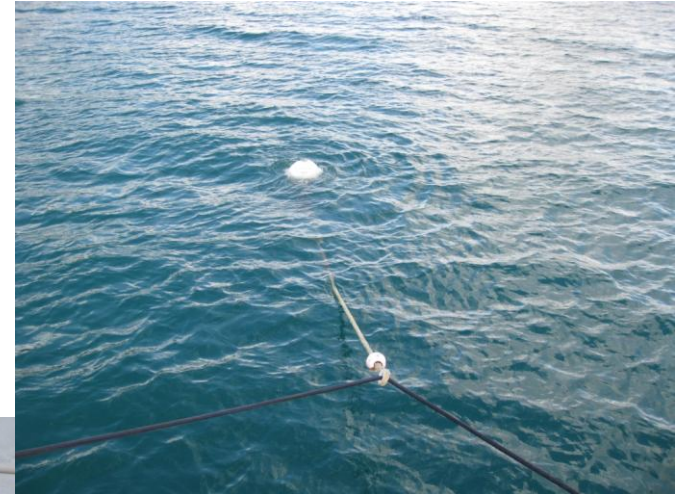
Moored with bridle from one bow cleat to the other bow cleat
