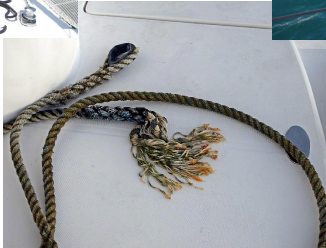
But, check the condition of the mooring line
